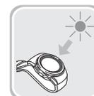
While you are wearing the watch, make sure that its LCD (solar panel) is not blocked from light by the sleeve of your clothing. Power generation efficiency is reduced even when the LCD is blocked only partially.
